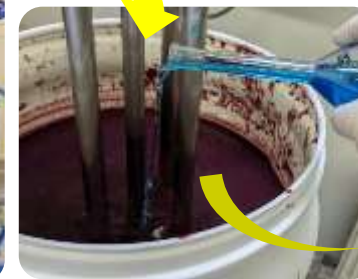
Spiked and homogenized (Silverson stirrer)
