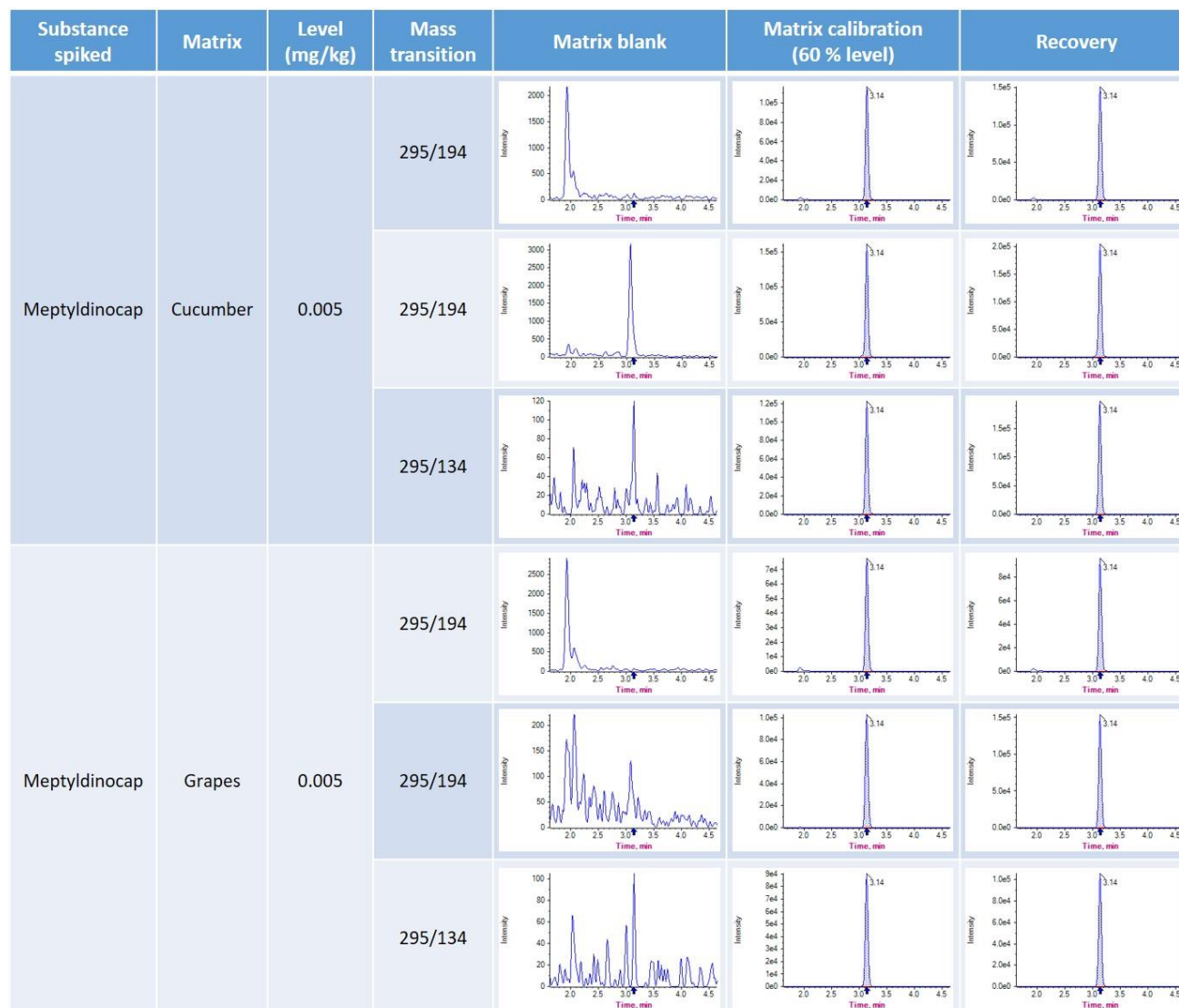
Figure 9: Selected chromatograms of the conducted validation of meptyldinocap following hydrolysis to 2,4-DNOP, in cucumber and grapes at 0.005 ppm. (The fast LC-method was employed)
