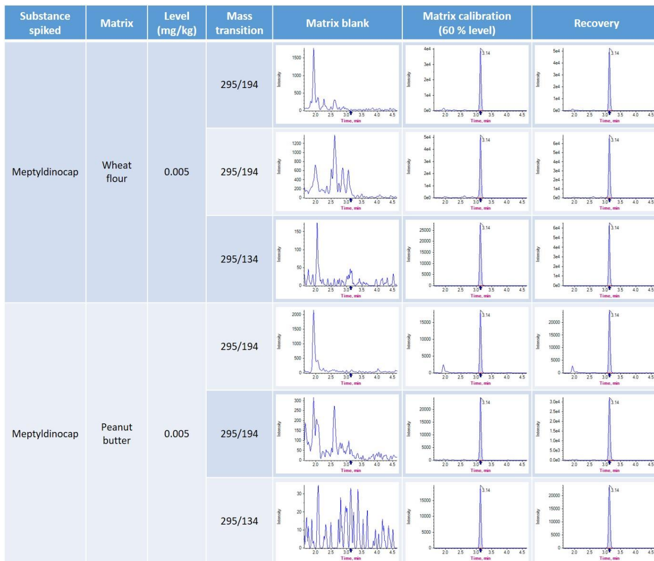
Figure 10: Selected chromatograms of the conducted validation of meptyldinocap following hydrolysis to 2,4-DNOP, in wheat flour and peanut butter at 0.005 ppm. (The fast LC-method was employed)
