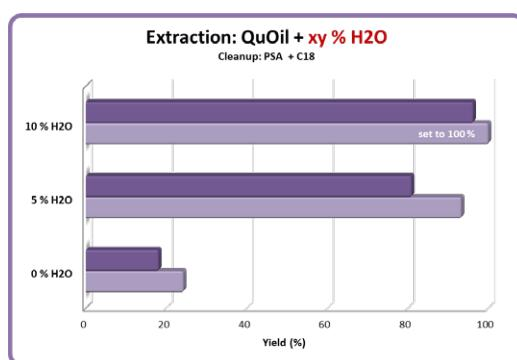
**Figure 4-2:** Impact of water addition and extraction time on the extractability of 2-CE
