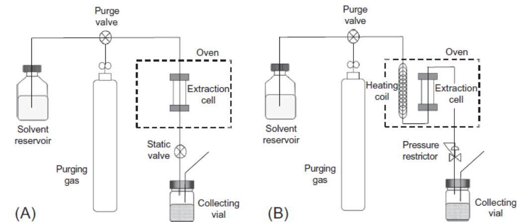
Fig. 13.1 Schematic PLE system. Configurations for development of (A) Static and (B) Dynamic PLE procedures.
