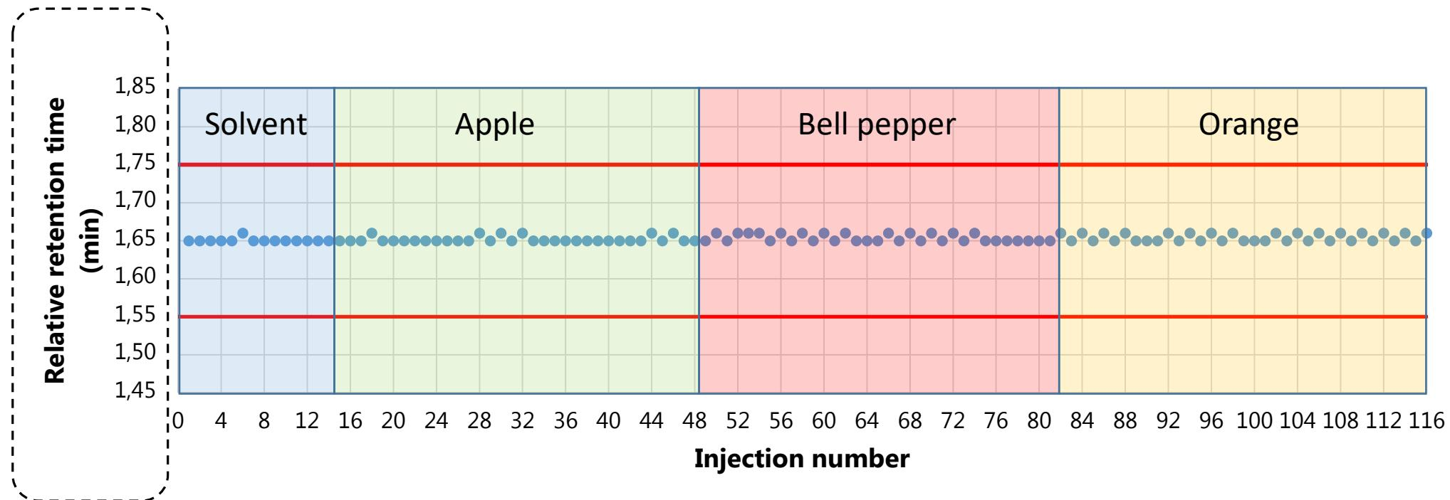
Retention time stability of pymetrozine. A sequence of 116 injections, alternate injections on channel 1 and channel 2. Red horizontal lines represent the  $\pm 0.1$  min tolerance specified in the DG SANTE Document.
