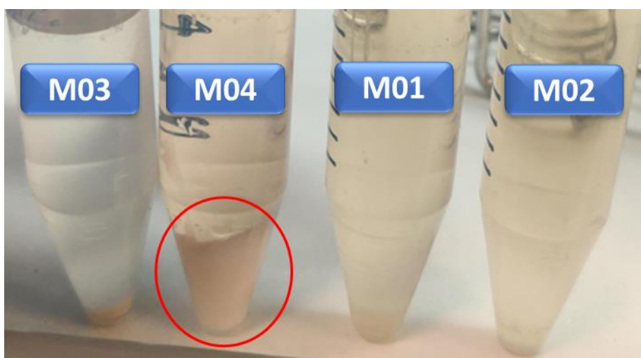
Figure 5. Extracts of white bean samples with the method M03, M04, M01 and M02, which includes a freezing-out step.
