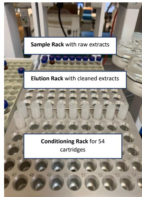
**Figure 3:** Robot used for automated sample treatment.
