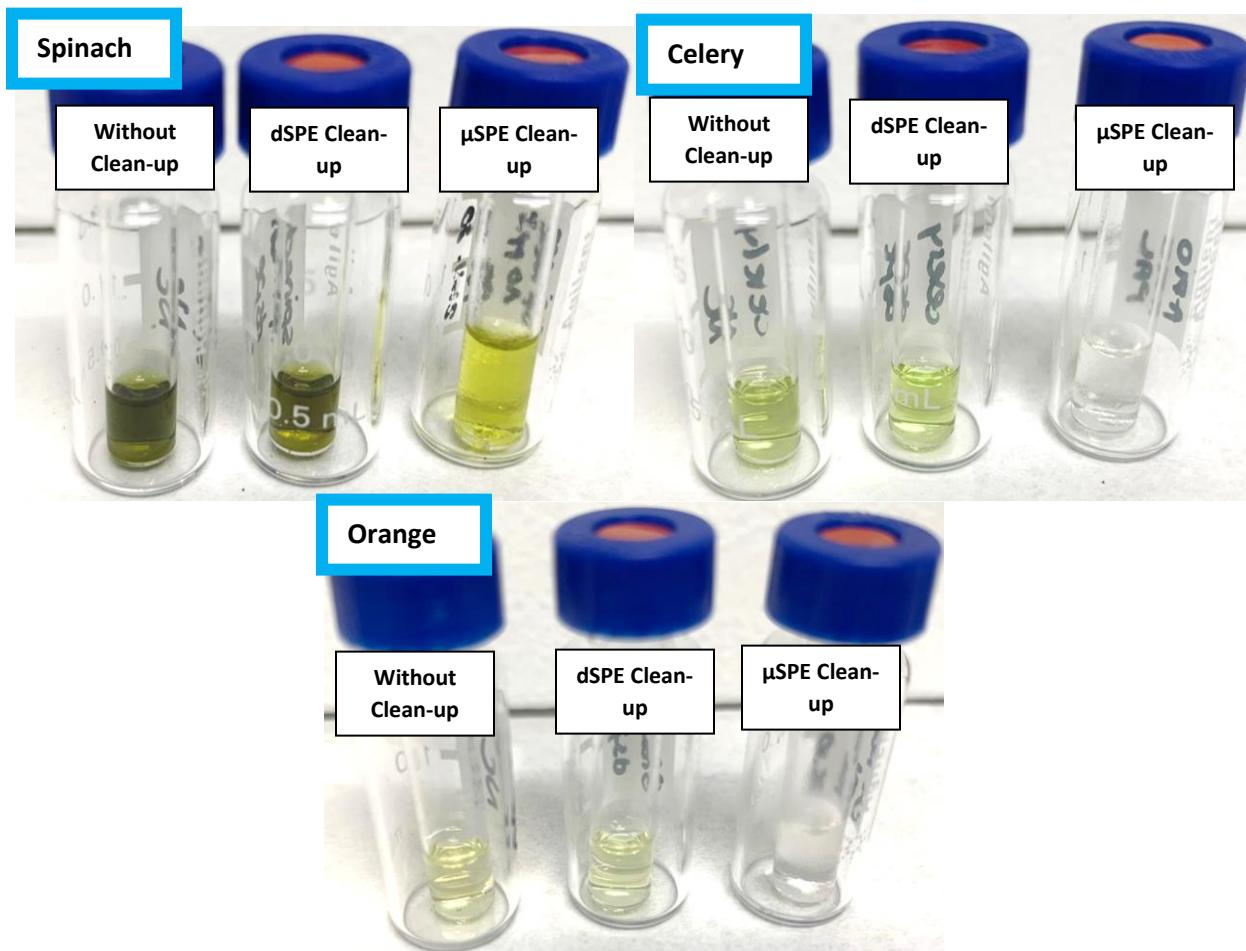
**Figure 8.** Extracts of spinach, celery, and orange. From left to right: raw QuEChERS extracts without clean-up, QC extracts (dispersive clean-up) and μSPE extracts (cartridges)
