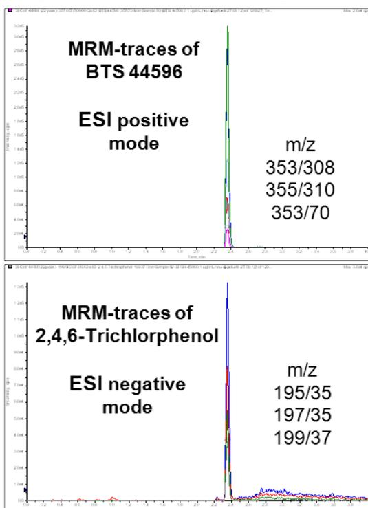
The chromatograms to the left demonstrate the in-source fragmentation of BTS 44596 to TCP. Injection of a fresh BTS 44596 solution resulted in a peak at the MRM-traces of TCP but at the retention time where BTS 44596 is expected rather than where TCP is expected. This indicates an in-source fragmentation of BTS 44596 to TCP. To ensure correct determination these two compounds they have to be separated chromatographically.
