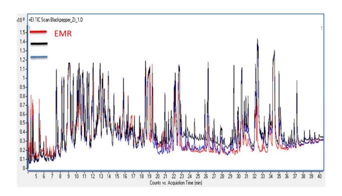
b) TIC of black pepper using EMR with 25 times total dilution (8x10<sup>7</sup> pg in column) and with and without freezing out.
