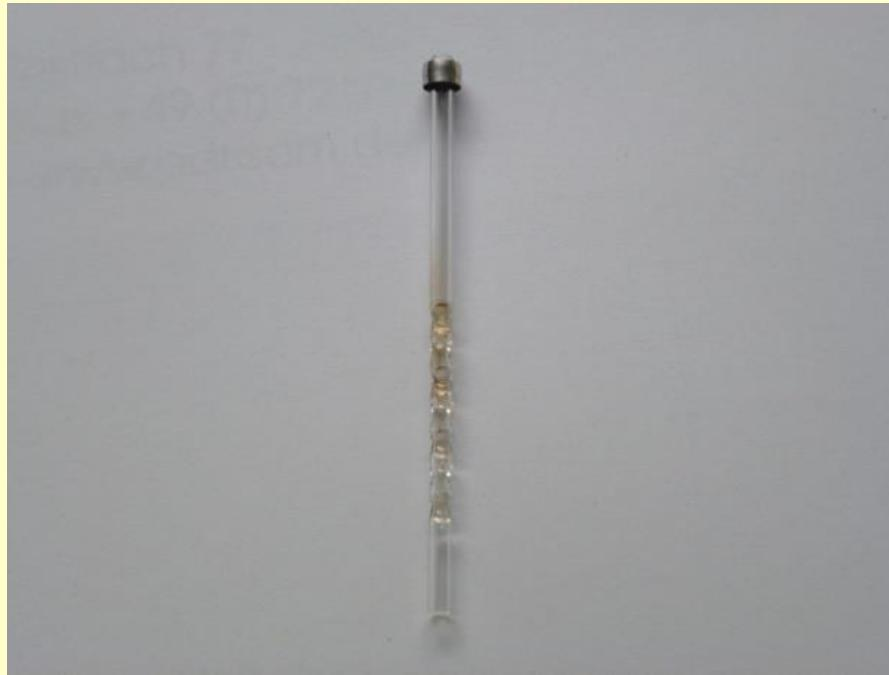
GC-Liner after tests and the liver validation study
