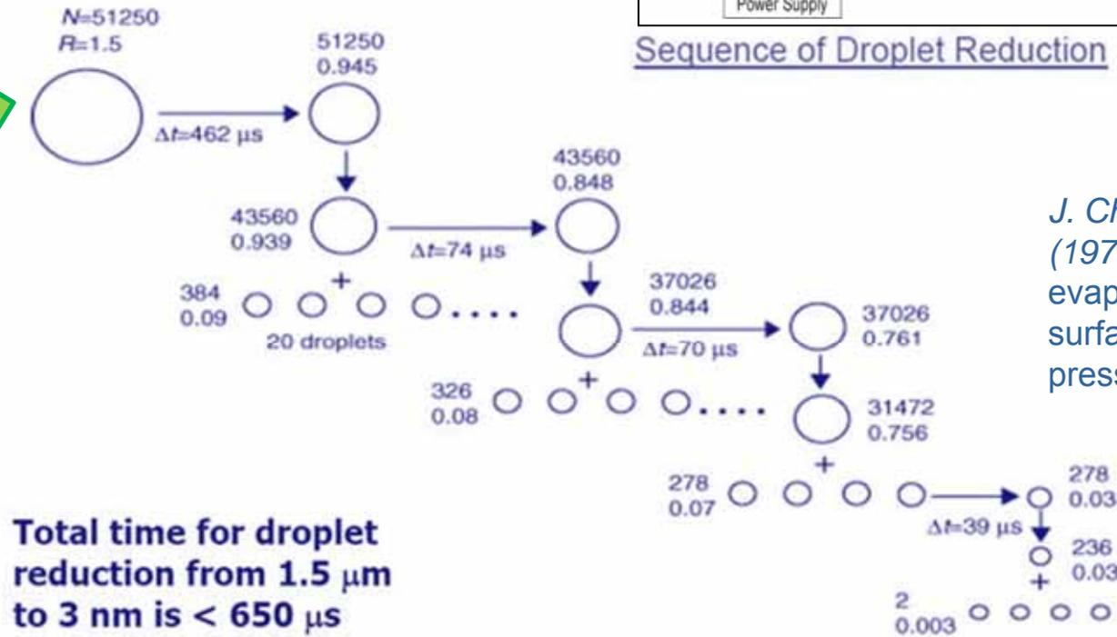
Total time for droplet reduction from 1.5  $\mu$ m to 3 nm is < 650  $\mu$ s
