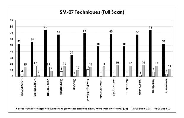
Chromatographic Techniques used in Full Scan to determine each pesticide in the test item
