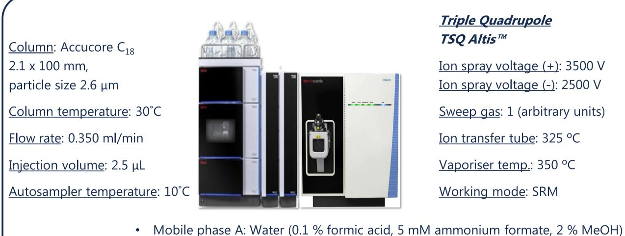
TSQ Altis™ <u>Ion spray voltage (+)</u>: 3500 V <u>Ion spray voltage (-)</u>: 2500 V Sweep gas: 1 (arbitrary units) <u>Ion transfer tube</u>: 325 °C
