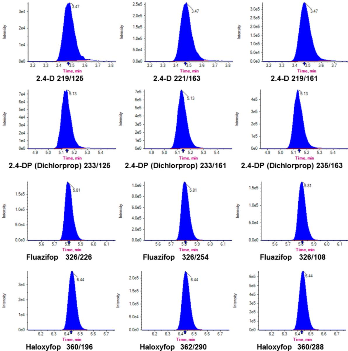
Fig 1: Chromatograms of 2,4-D, Dichlorprop, Fluazifop, Haloxyfop 0.1 µg/mL in Acetonitrile.
