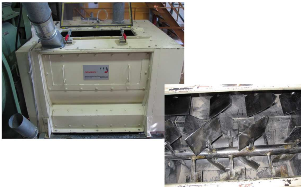
Dinnissen twin-shaft paddle mixer type 300 L
