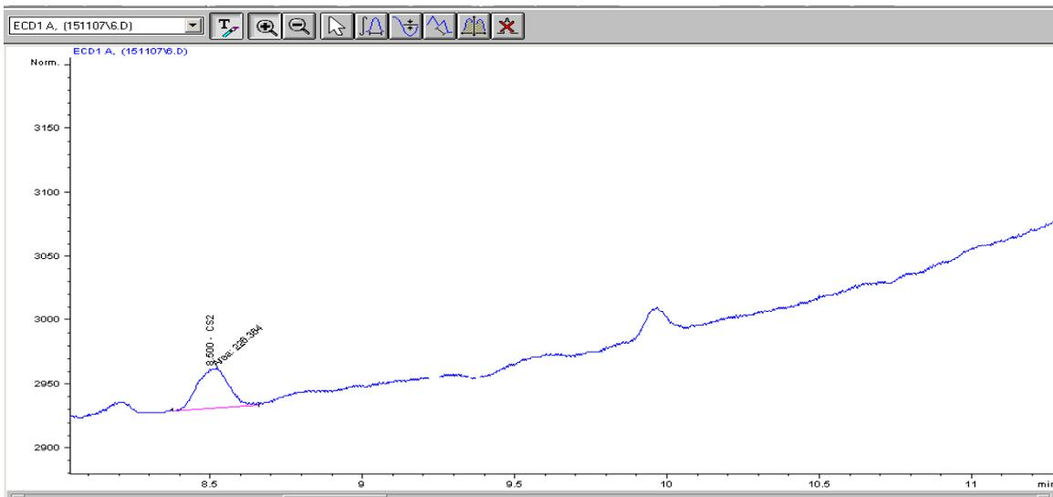
**Fig.3: cucumber sample with 0.20 mg/kg CS<sub>2</sub>**
